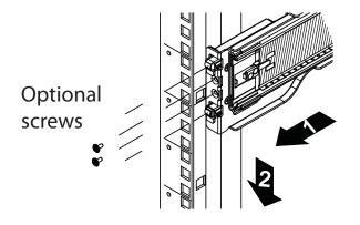
8 Repeat Step 7 to mount the four ends, extending the rails as necessary.
